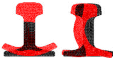
Figure 1: Example of guided wave mode shapes with energy concentrated in the foot (left) and web (right) of the rail respectively.
